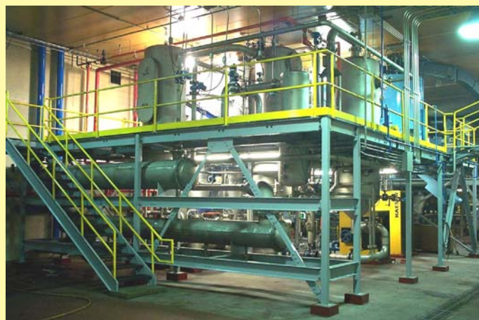
Figure 3: Ensyn Transported Bed fast pyrolysis plant at Red Arrow, USA
