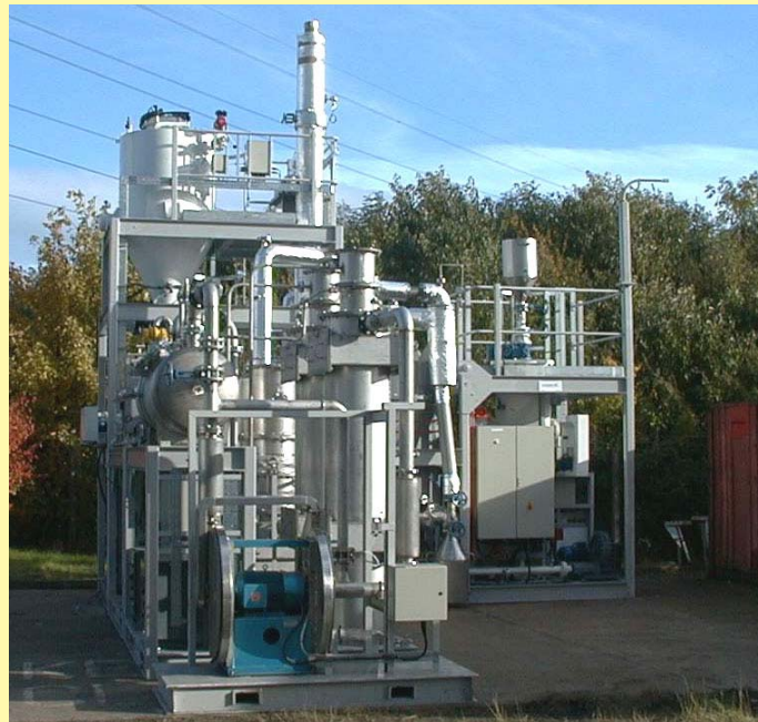
Figure 2: Fluid bed fast pyrolysis plant at Wellman, United Kingdom
