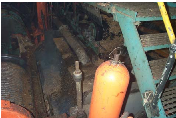
Pict. 14: The juice extraction rollers
