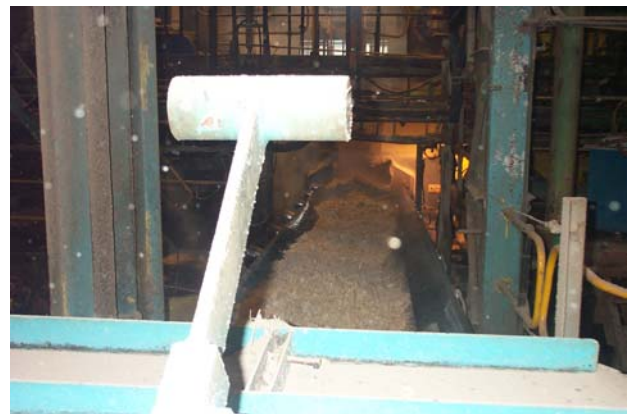
Pict. 17: Bagasse feeding to intermediate storage
