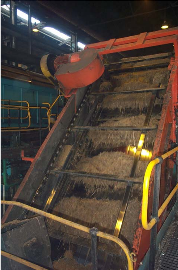
Pict. 13: Milled sugar cane feeding to extraction
