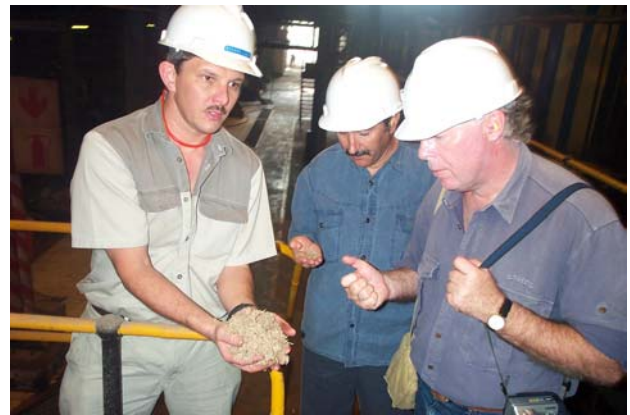
Pict. 16: Sugar cane after juice extraction - fibrous bagasse
