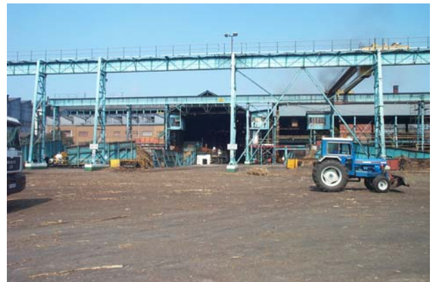
Pict. 11: Feeding to the two sugar lines – left the diffusion and right the milling line
