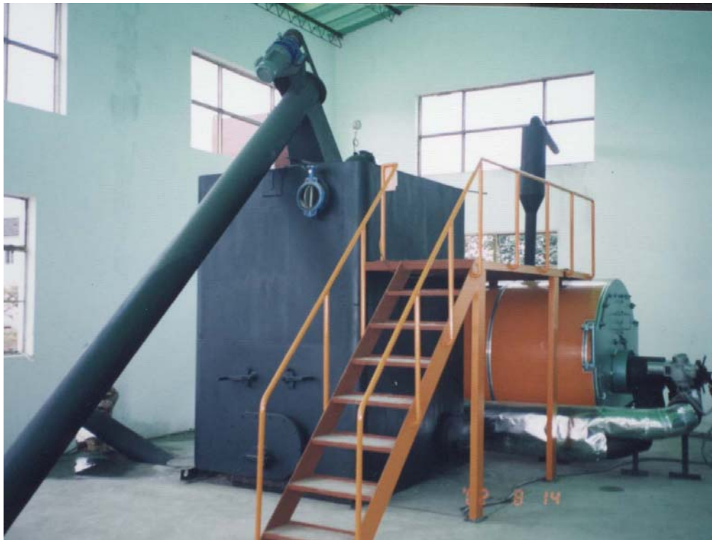
Photo of 1.4MW straw gasification-heating set
