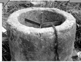
Small biogas reactor for 1 household
