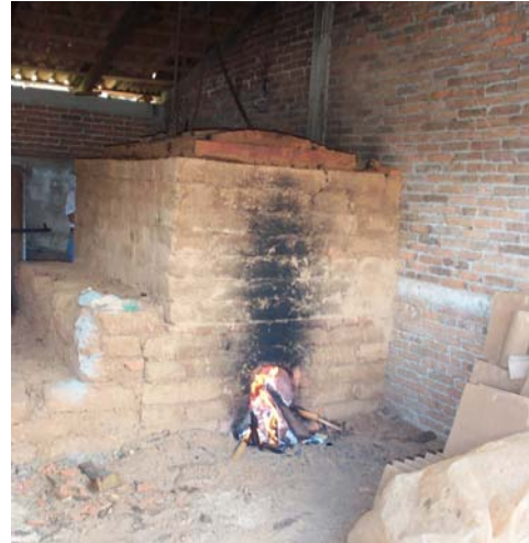
At Napízaro the tour visited the brick making enterprise 'Industrias Mendiola'. Tour participants were provided with an insight into the process of brick and tile making, from the extraction of raw materials to the end products. The bricks and tiles are dried in traditional wood fuelled ovens.
