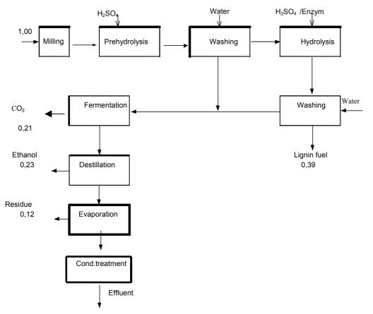
Figure 2. Schematic process design of ethanol production from wood. Figures in ton per odt (ton dry matter) raw material.
