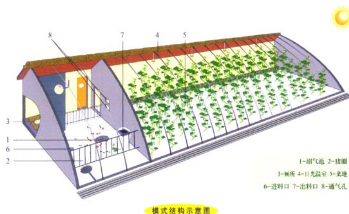
Figure 1: 'Four-in-one' biogas model for Northern China
