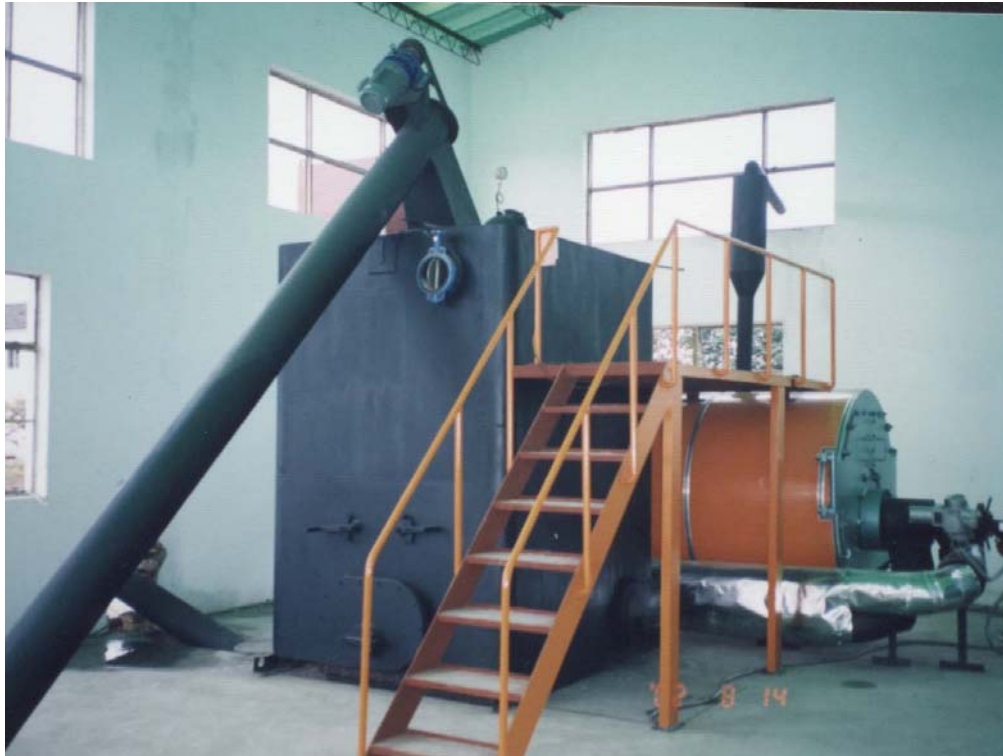
Photo of 1.4MW straw gasification-heating set
