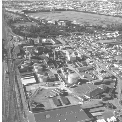
Figure 3: Merebank downstream plant near Durban, South Africa, with an ethyl alcohol production capacity of 40 million litres per year (Source: Illovo Sugar Ltd, South Africa)
