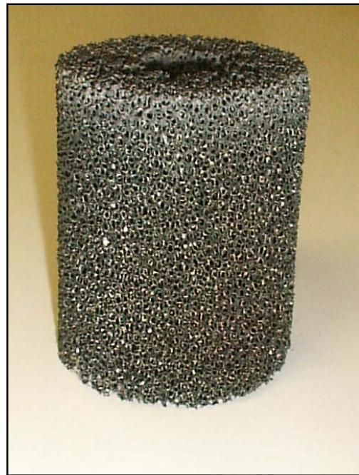
Figure 4.1: Ceramic body of the porous burner
