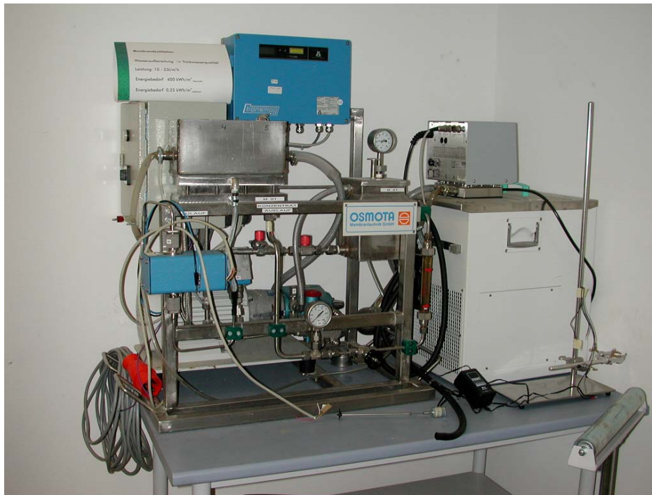
Figure 7: Experimental plant of membrane distillation
